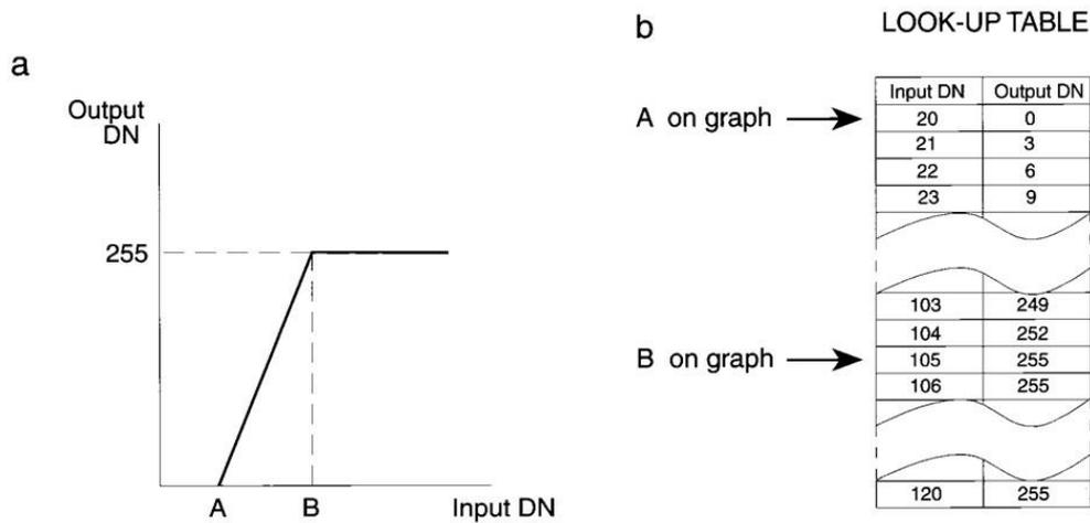
Fig. 12 (a) A sample linear transformation function used for contrast stretching (b) LUT for this function
