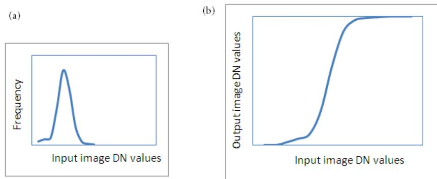
Fig.5 (a) Sample histogram of an image and (b) Function used for histogram equalized stretch For example, for an 8-bit display system, the histogram equalization function used for stretching the input image can be represented as follows.
