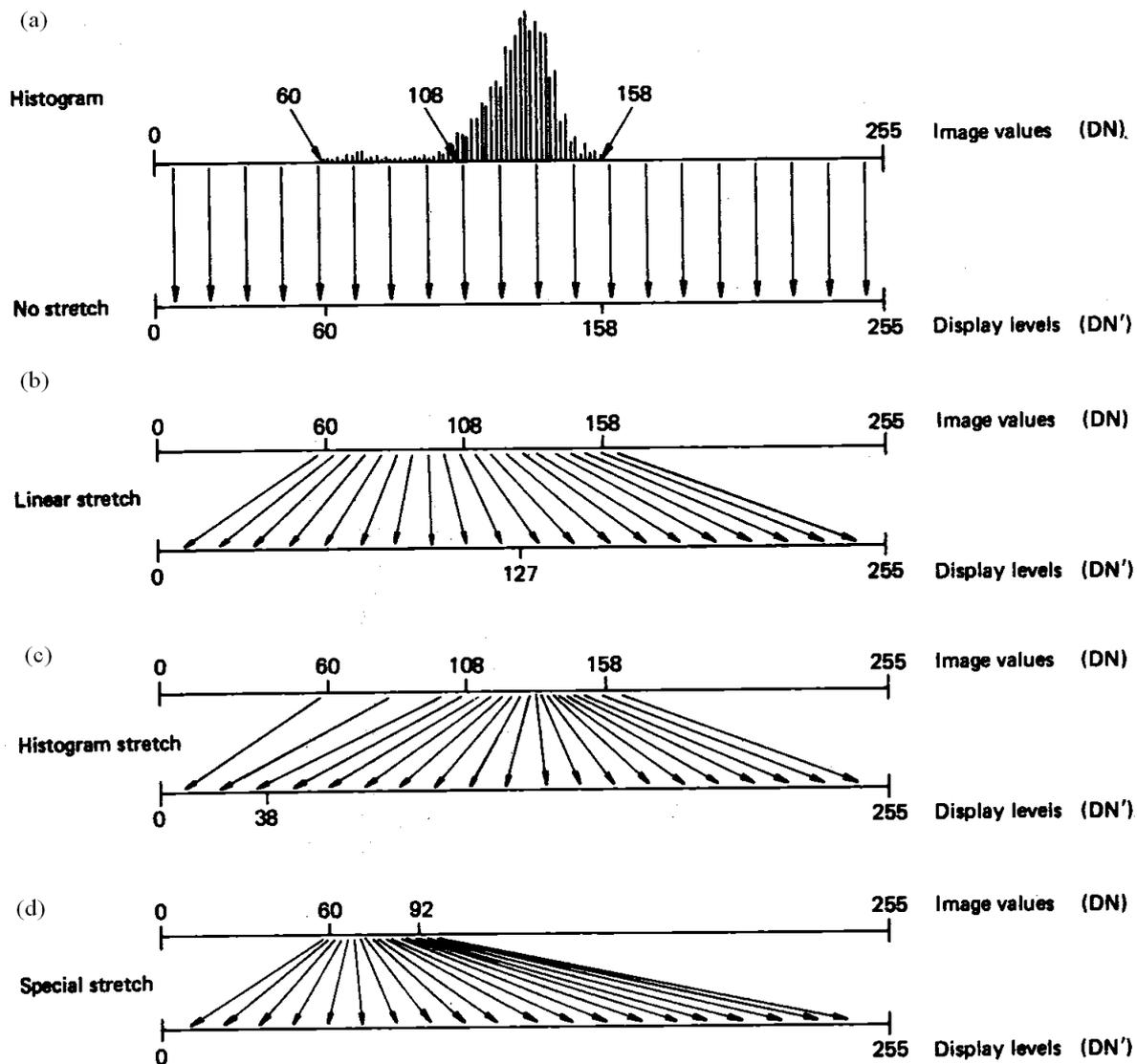
Fig. 11. Schematic representation showing various contrast stretching algorithms (Courtesy: Lillesand et al., 2004)
