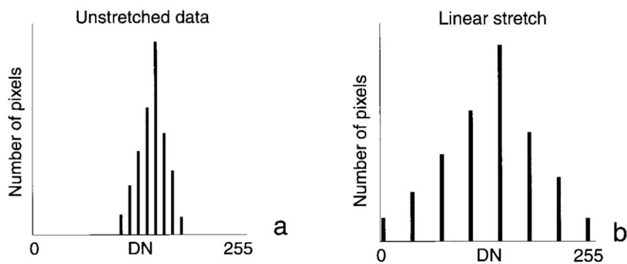
Fig. 3 Histograms of the Landsat TM Band-5 image before and after contrast stretching
