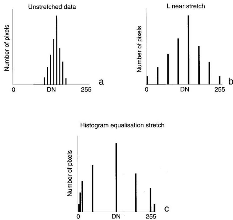
Fig. 4. Histograms of (a) Unstretched image (b) Linear contrast stretched image(c) Histogram equalised image Fig.5 (a) shows a sample histogram of an image and Fig.5 (b) shows the corresponding histogram-equalization stretch function. Input DN values corresponding to the peak of the histogram are stretched to a wider range as shown in the figure.
