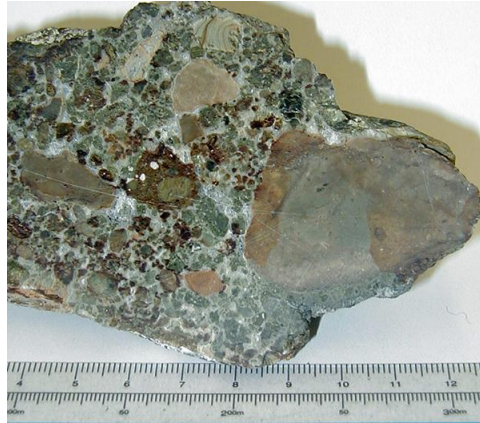
Figure 3- Hypabyssal facies kimberlite. The white matrix is calcite while the green material is serpentine.
