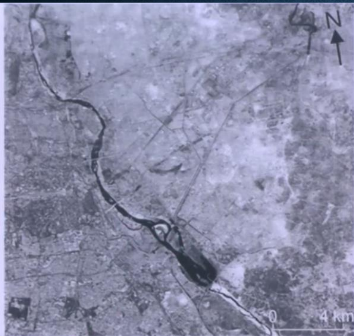
Figure 3. Showing IRS-IC-PAN image of 11 February 1997 of New Delhi, the national capital of India and surroundings. This image has been used as master image for image-to-image transformation and later as intensity image during the final stage of IHS-to-RGB transformation.
