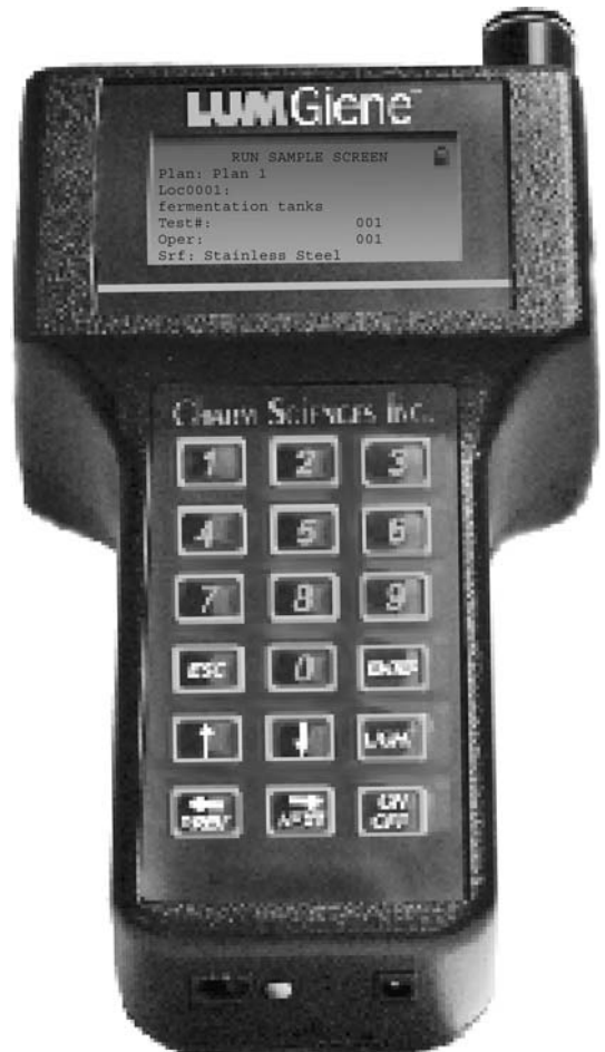
Figure 3–4 Device for the rapid determination of hygienic conditions.
